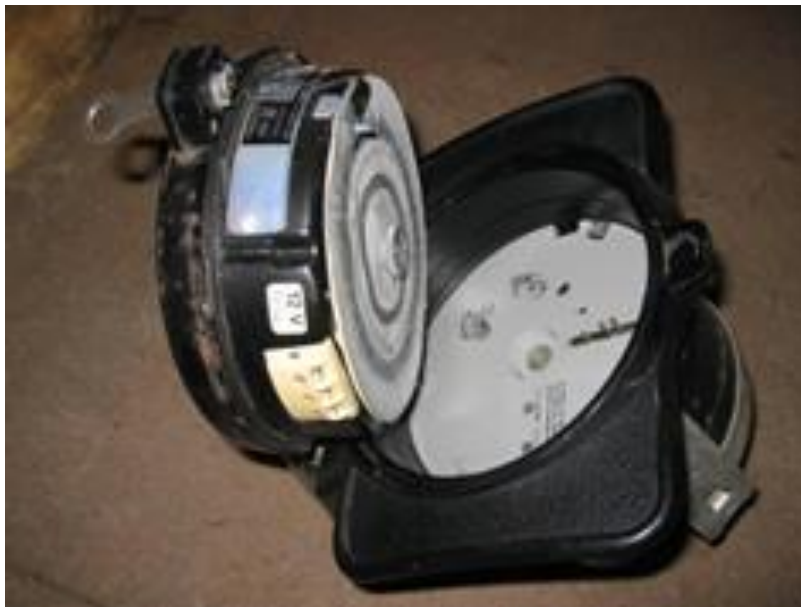
Figure 3.1.3-1. Mechanical tachograph with paper chart displayed
