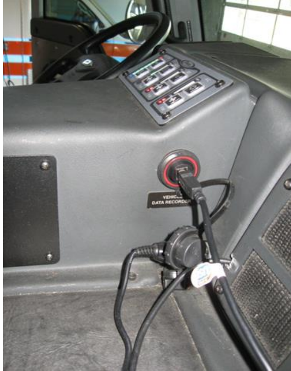
Figure 3.4.2-3. NFA 1901 USB type-A connection port
