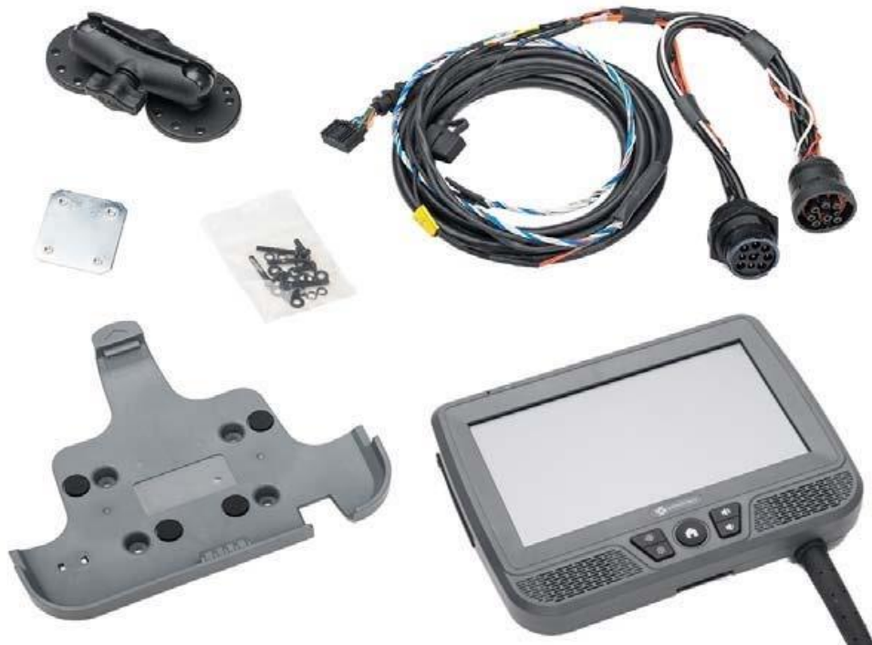
Figure 3.2.1.2-2. Omnitrac's IVG interconnecting hardware 23
