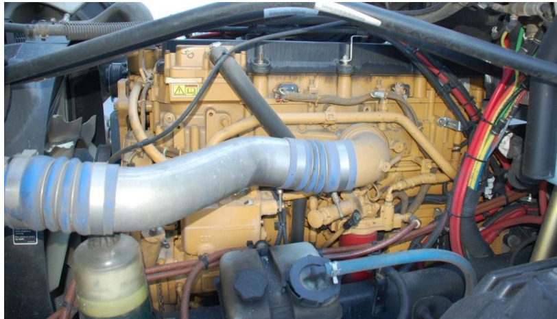
Figure 3.1.3-1. Typical Caterpillar engine ECU location
