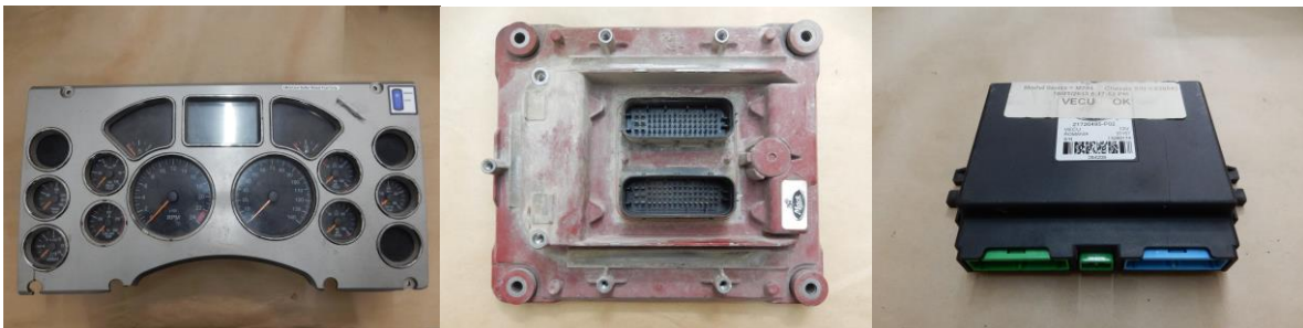
Figure 3.1.4-2. V-MAC IV IPECU (left), EECU (middle) and VECU (right)
