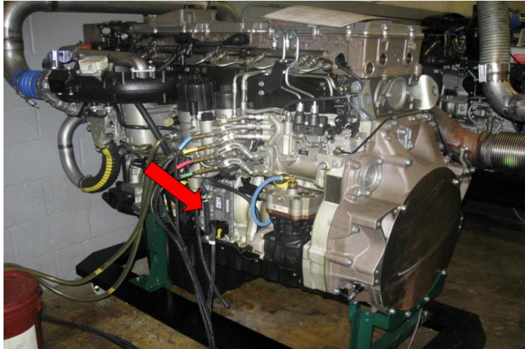
Figure 3.1.1.1-2. Typical DDEC VI/10/13/16 MCM location
