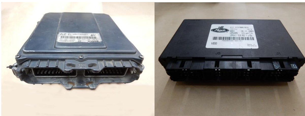
Figure 3.1.4-1. V-MAC III EECU (left) and VECU (right)
