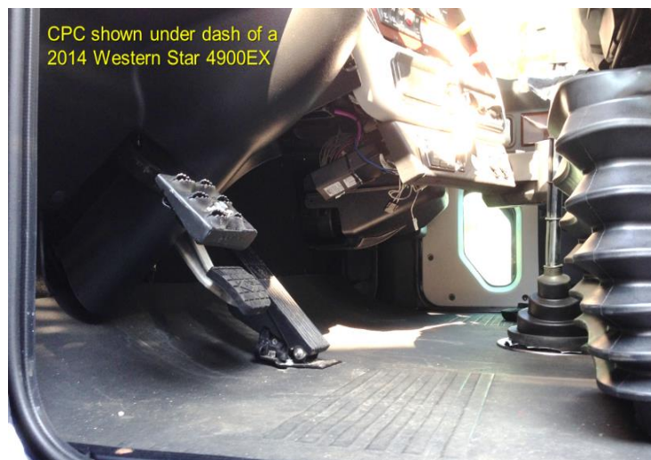
Figure 3.1.1.1-1. Daimler CPC ECU, 2014 Western Star
