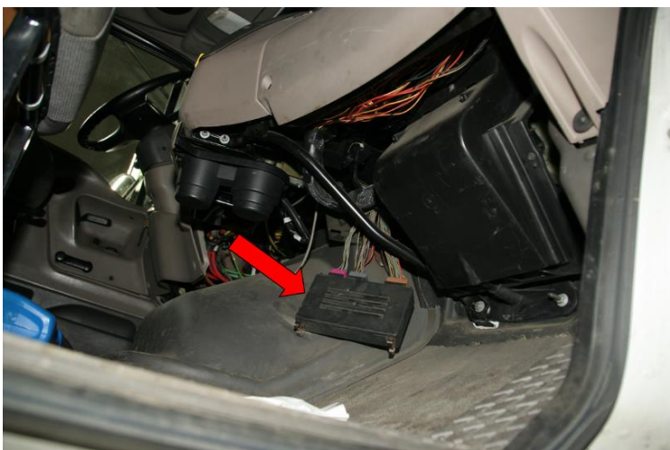
Figure 3.1.1.2-2. Typical MBE VCU location
