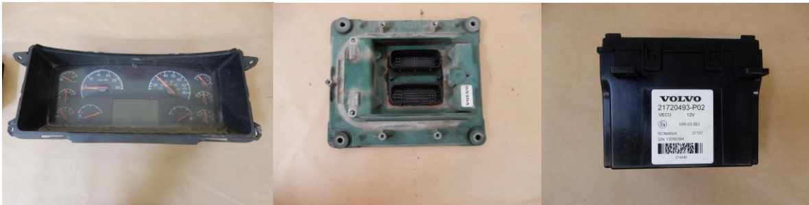
Figure 3.1.5. Ver. 2/Ver. 3 IPECU (left), EECU (middle) and VECU (right)
